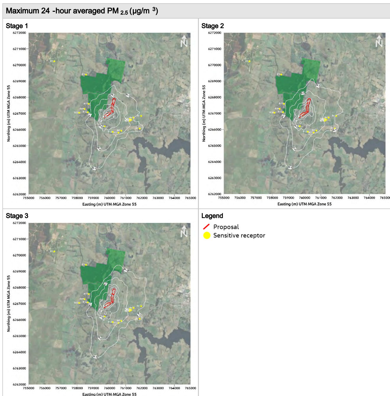
Figure 6.4. Ground-level concentration contours, proposal maximum 24 -hour averaged PM 2.5 contributions
